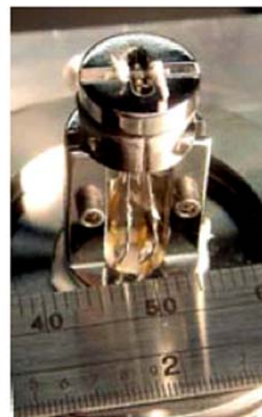
FIGURE 7 (a) Schematic of a QCL based QEPAS sensor platform showing a QTF and acoustic micro-resonator. (b) Picture of a QEPAS absorption detection module consisting of a QTF and micro-resonator
