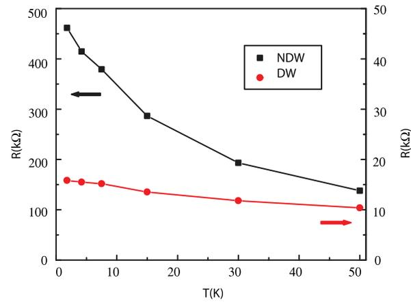
**Extended Data Figure 3 | Temperature-dependent electrical transport through bulk bilayer graphene and through the AB-BA domain wall.** The CNP resistance ( $V_{\text{bg}} = -140$  V) of a bilayer graphene device without a domain wall (NDW, black line) increases by over  $300 \text{ k}\Omega$  ( $\sim 2.5$  times) as the temperature is decreased from 50 K to 1.8 K. In contrast, the CNP resistance
