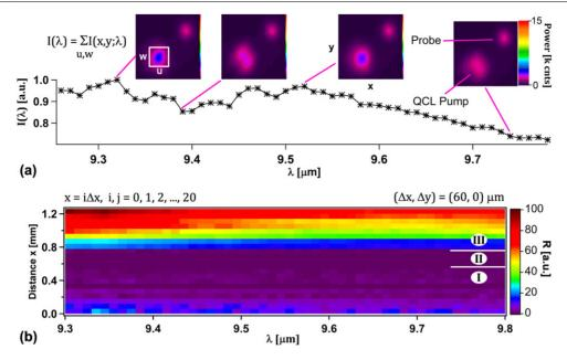
**Figure 3.** (*a*) The QCL energy  $I(\lambda)$  and selected beam profiles revealing the QCL modes. The probe beam is offset for illustration purposes. (*b*) Spectra  $s_{ij}$  for a fixed j and i = 1, 2, ..., 20 scanning over black enamel paint (I), Al substrate (II), purple cosmetic paint (III).
