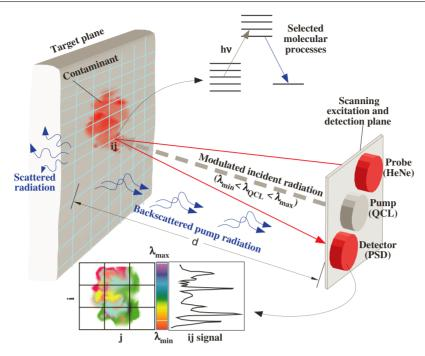
**Figure 1.** The concept of pump–probe standoff hyperspectral imaging using QCL-based photothermal spectroscopy of a target surface. The modulated QCL pump thermo-optically stimulates the surface via an available molecular channel. The minimally invasive probe beam (red) impinging on the same exposed surface location monitors the thermal response of the specimen, which yields the absorption spectra of the molecular composition of the target.
