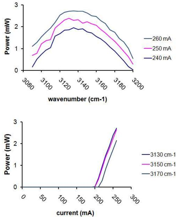
Fig. 6. Power vs. wavelength (top panel) and power vs. injection current (bottom panel) for ECiL at 15°C.
