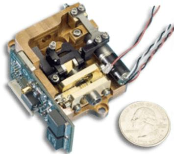
Fig. 4. Photograph of the Daylight Solutions external-cavity broadly tunable interband-cascade laser source.
