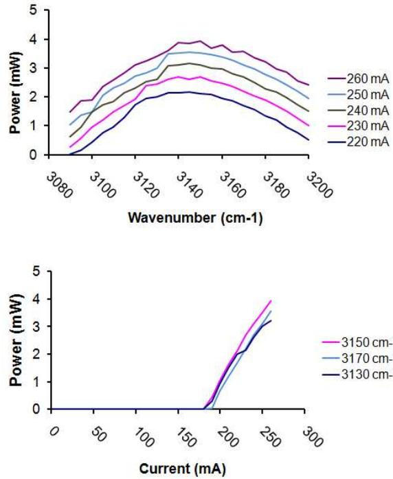
Fig. 5. Power vs. wavelength (top panel) and power vs. injection current (bottom panel) for ECiL at 10°C.
