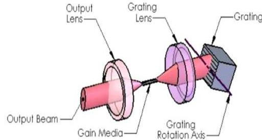
Fig. 3. Schematic representation of the main components of an external cavity interband cascade laser.
