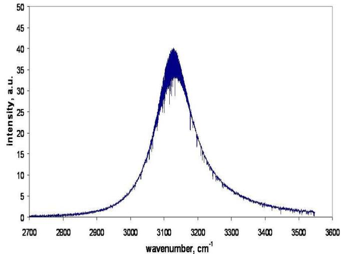
Fig. 2. FTIR spectrum of ASE from the Fabry-Perot ICL at 125 mA and 15°C.
