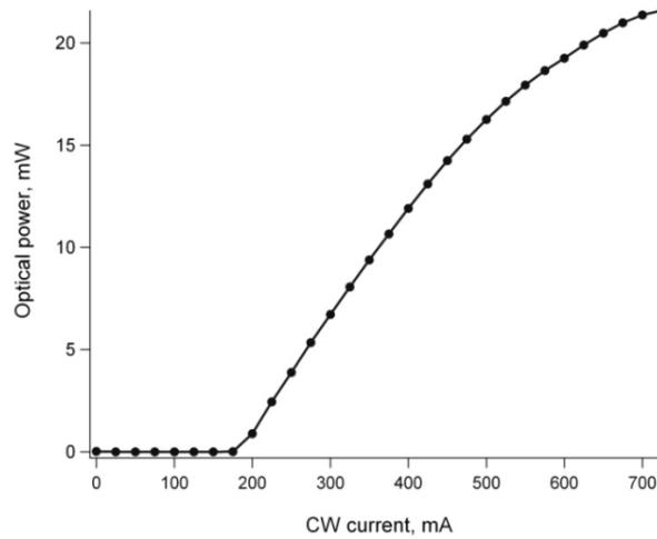
Fig. 1. CW  $P$ - $I$  curve for the uncoated ICL chip at 15°C.
