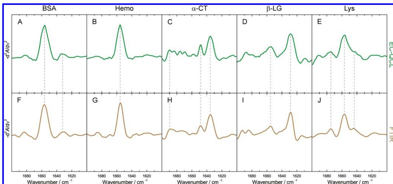
**Figure 4.** Inverted second derivative spectra of sample proteins acquired by the EC-QCL setup (A–E) and FT-IR spectroscopy (F–J). Gray dashed lines highlight the high overlap of the spectral features between the IR spectra acquired by EC-QCL and FT-IR spectroscopy.
