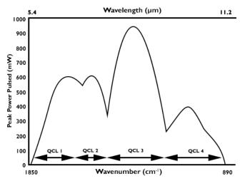
Tune > 1,000 cm<sup>-1</sup> in 100 ms (example tuning curve for MIRcat-2400-PX-B configuration shown)
